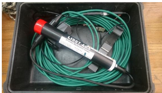
Figure 2.87. Acoustic sensor LISST-ABS.
