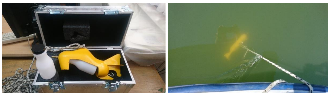
Figure 2.86. Isokinetic physical drift catcher DH-59.
