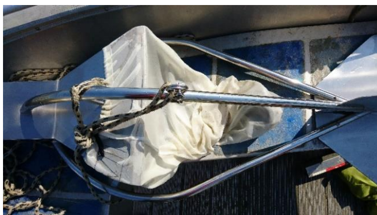
Figure 2.88. Helley-Smith type trailed sediment catcher.
