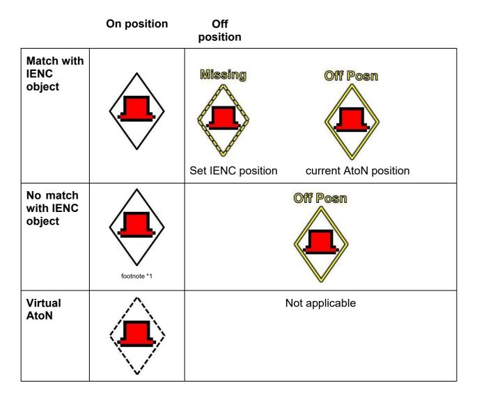
\*1 If there is an AtoN object without MMSI in the IENC it is not possible to match the two objects. The AIS AtoN symbol will be displayed in addition to the IENC object in this case. In case both objects are not very close they are displayed next to each other.
