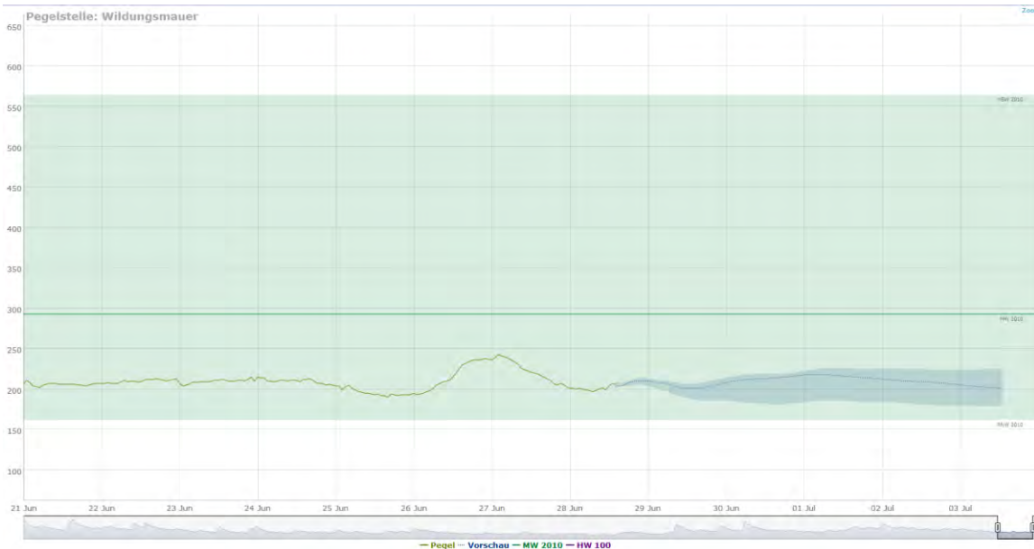
Figure 16: Example of a water level visualisation of a gauge
